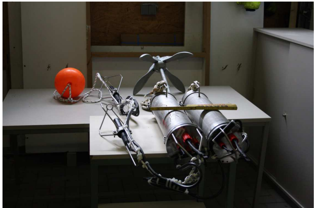
Figure B.1 Overview of ITAP system, two recorders with each its own hydrophone.
